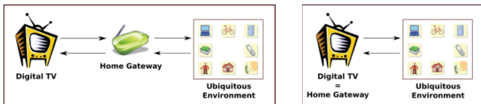
(a) Digital TV interacts with an ubiquitous environment through a Home Gateway
